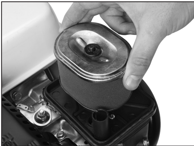
Figure 21. Removing the air filter.
